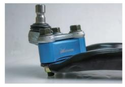
RC Adjuster is good for lowered vehicle; it is able to correct the angle of front lower arm to factory setting and prolong the life time of arms and ball joints. 三角架墊片功用是改善三角架水平位置,讓更改避震器降低車高設定的車輛,可提升懸 吊轉向幾何位置關係,讓和尚頭及三角架鐵套壽命更長、更耐用
