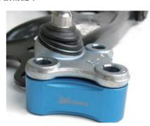
1. Remove three bolts from ball joint. 安裝前須把三角架和尚頭3支固定螺絲取下
